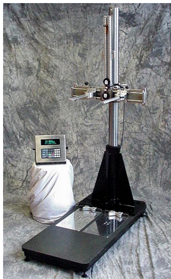
Figure 3. The Anatometer The Anatometer measures postural asymmetry and was designed to decrease the number of radiographs required in patient care.
